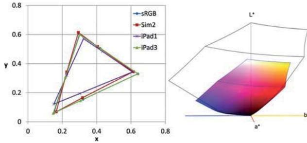
**Fig. 7.** Left: Gamut in x-y coordinates: Sim2 (red) compared to typical displays (iPad1 (violet), iPad3 (green)); sRGB gamut is almost identical to iPad3 gamut. Right: Gamut in CIELAB coordinates: Sim2 (grid) with iPad3 (colored).
