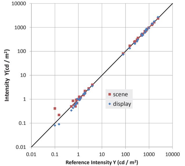
**Fig. 6.** Measured lightness range for display and scene compared to intensities in HDR image.
